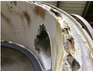
O ring groove after initial abrasive blast
